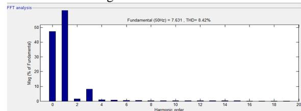
Fig.15. THD level of Load current
