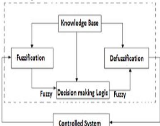
Fig.6. Basic structure of Fuzzy Logic controller
