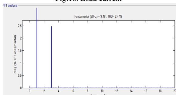
Fig.19. THD level of Load current
