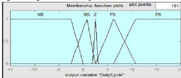
Fig.9 Output variables to defuzzification process
