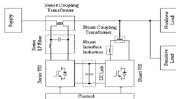
Fig.2. Schematic diagram of Unified Power Quality Conditioner
