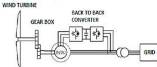
Fig.1. Grid connected DFIG based wind power system
