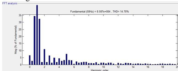
Fig.12. THD of Load current waveform
