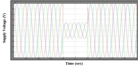
Fig.10. Voltage sag due to three phase to ground fault
