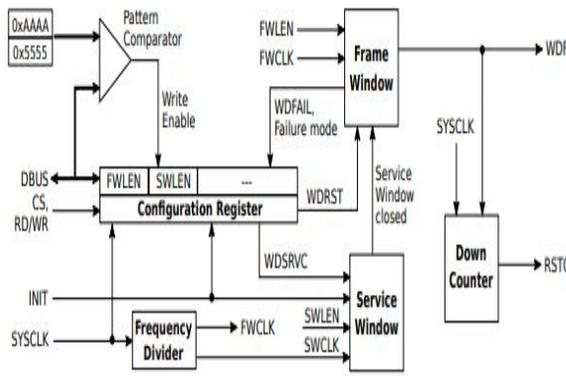
Fig. 6. Functional block diagram of the proposed watchdog timer
