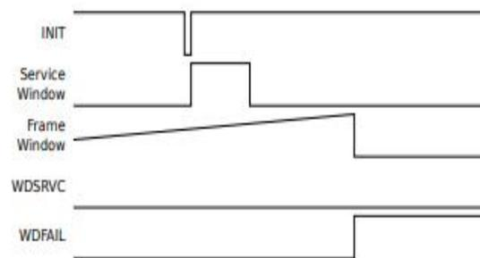
Fig. 3. Watchdog fail due to frame window expiry
