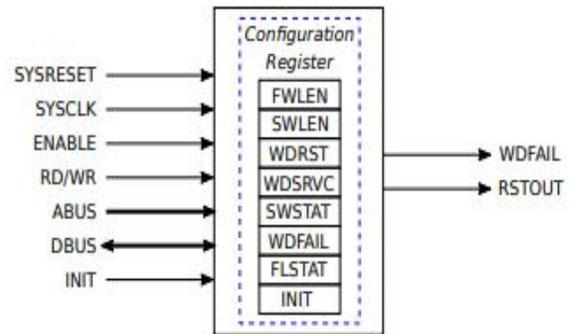
Fig. 1. Watchdog timer input-output interface and configuration register
