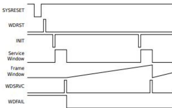
Fig. 2. Watchdog timer initialization and service operation
