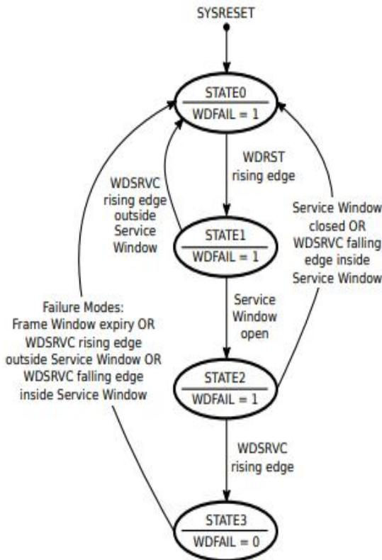
Fig. 7. Finite state machine design of watchdog fault detection logic
