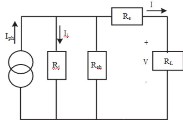
Fig.2 Equivalent circuit of PV array
