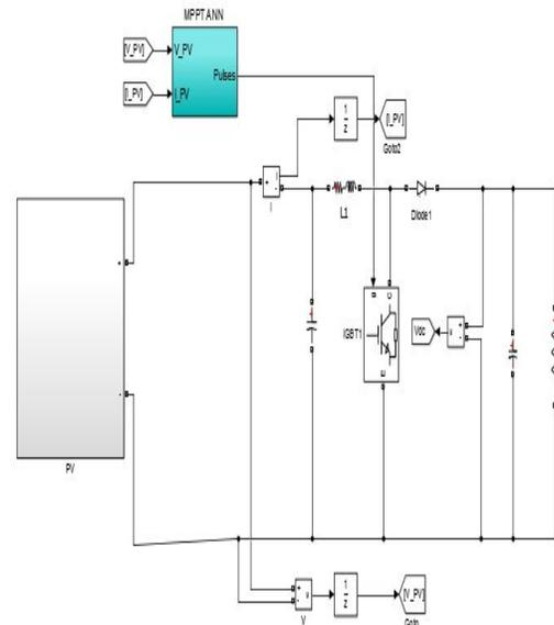
Simulink diagram for proposed system
