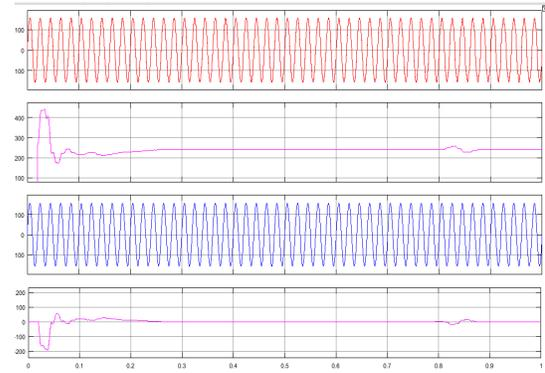
Fig. 9 Simulation waveforms before and after grid distortion. (a) Results of PLL. (b) Results of active and reactive power of ES system
