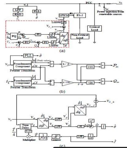
Fig. 3 The proposed power control of ES-2. a) Control diagram. (b) Calculation diagram of active and reactive power. (c) Functions of PLL and harmonic extraction.
