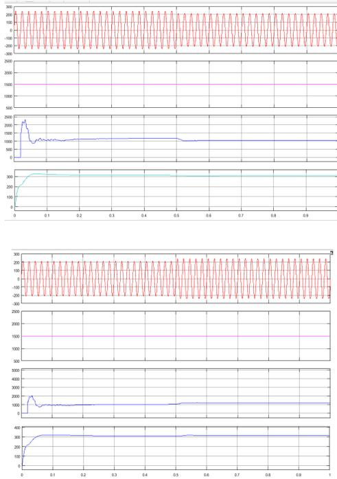
Fig. 8 Transient ES-2 responses to a change of the line voltage with  $P_{inref}=1.5kW$ . (a) From 240V to 210V. (b) From 210V to 240V.
