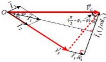
Fig. 4 Vector diagram of ES-2 circuit with resistive CL.
