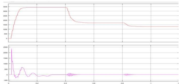
**Fig. 7 Simulation waveforms under different variations of the input active power. (a) From 1.6kW to 1.1kW and then back to 1.6kW @  $V_G=230V$ . (b) From 8kW to 2kW and then back to 8kW @  $V_G=200V$ . (c) From 8kW to 4kW and then to 2kW @  $V_G=200V$ .**
