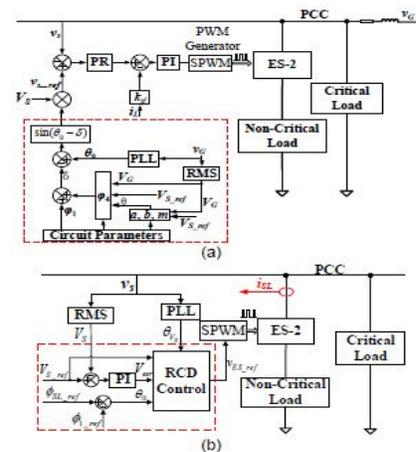
Fig. 2 ES-2 control diagrams for (a)  $\delta$  control, (b) RCD control.
