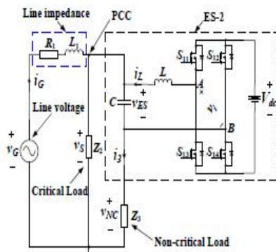
Fig. 1 Topology of ES-2 and associated circuitry.
