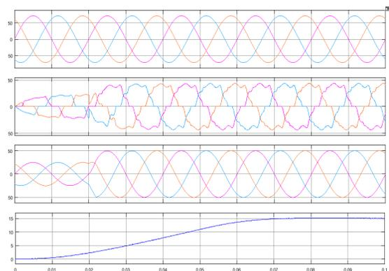
Fig:9 (a) Source voltage. (b) Transient response of the load current before compensation. (c) Transient response of the source current after compensation (d) DC-link voltage.
