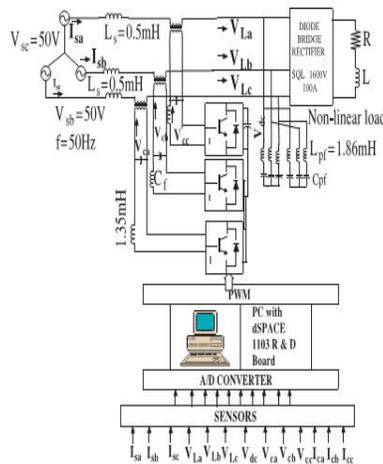
Fig. 1 Schematic diagram of the control and power circuit of the HSAPF
