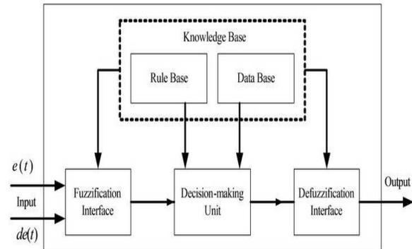
Fig. 3 Architecture of Fuzzy Logic Controller
