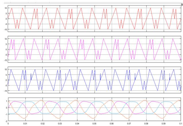
Fig 8 : Three-phase compensating voltages and Load voltage after compensation for fuzzy logic controller-based HSAPF system.
