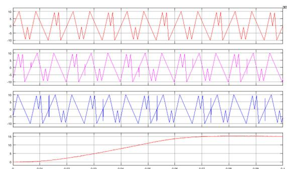
Fig:10 Three-phase compensating voltages and dc link voltage for fuzzy logic controller-based HSAPF system.
