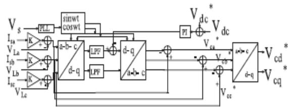
Fig. 2. Reference generation scheme (HSRF).
