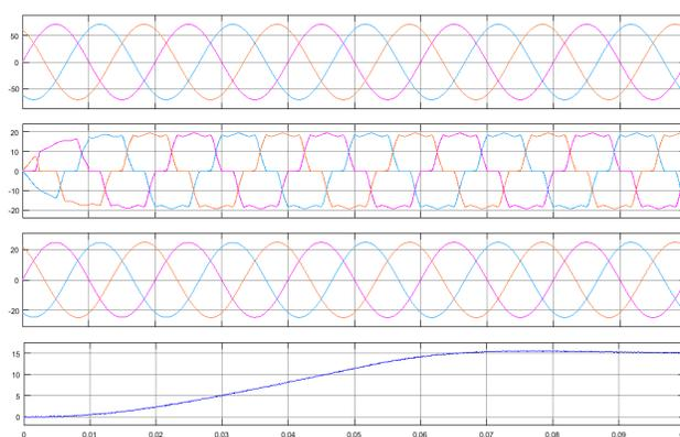
Fig 7 (a) Source voltage(b) Steady-state response of the load current before compensation(c) Steady-state response of the source current after compensation(d) DC-link voltage.
