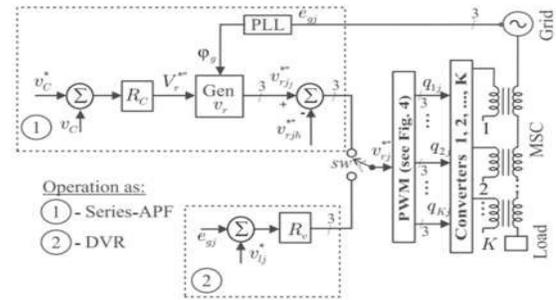
As shown in Fig. 7, the switch SW indicates the selection of Series-APF or DVR operation.
