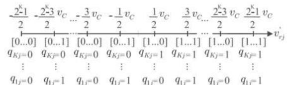
Fig. 5. One-dimension of output voltage ( $v_{rj}$ ) levels region for  $K$ -stages (i.e., that means  $N_1 = 1, N_2 = 2, N_3 = 4, \dots, N_k = 2(K - 1)$ ).
