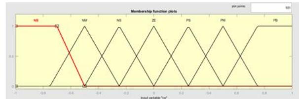
Figure 10: cumulative Error Input Membership Function
