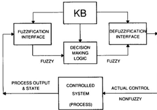
Fig. 8. Basic configuration of fuzzy logic controller (FLC). In this section, we present the main ideas underlying the FLC.
