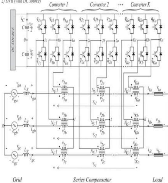
Fig. 1. Proposed MSC. Generalization with K-stages (i.e., K-cascaded transformers and K-TPB converters)
