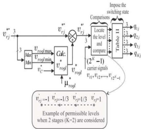
Fig. 7. Control block diagram of proposed MSC. Possible operations as a Series-APF (option 1) or as a DVR (option 2).
