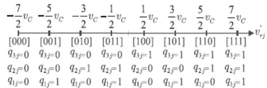
Fig. 4. One-dimension of output voltage ( $v_{rj}$ ) levels region for three-stages (i.e.,  $K = 3$  that means  $N_1 = 1, N_2 = 2,$  and  $N_3 = 4$ ).
