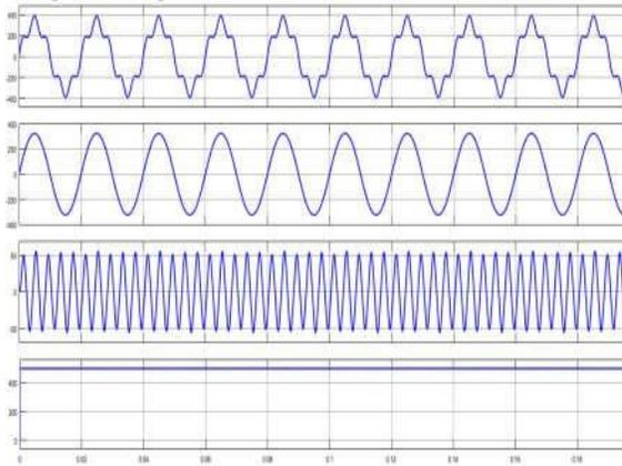
Fig. 9.Simulation result.MSC operating as a Series-APF. System voltages and the regulated dc-link voltage
