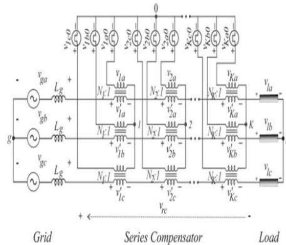
Fig. 2. Ideal equivalent circuit for generalization of the proposed MSC
