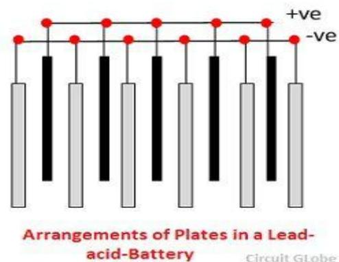
**Fig: Arrangements of plates in a lead acid battery**
