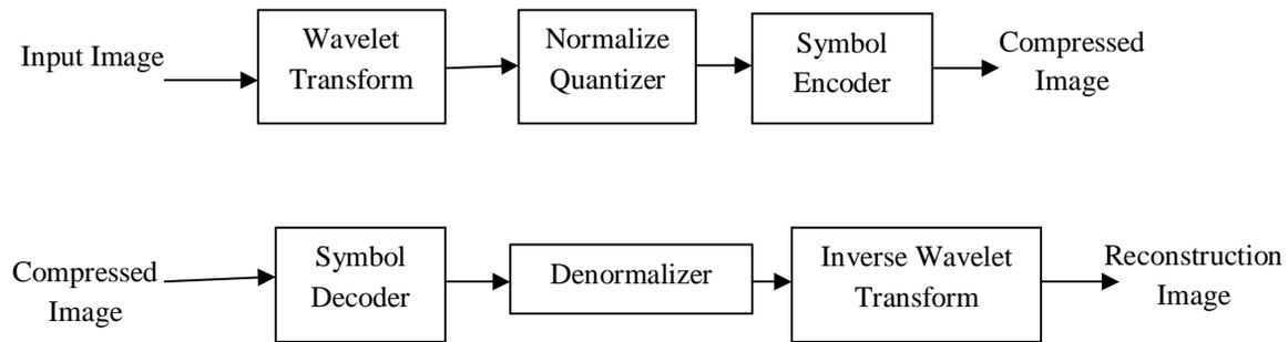
**Fig.4: Image compression using wavelets**
