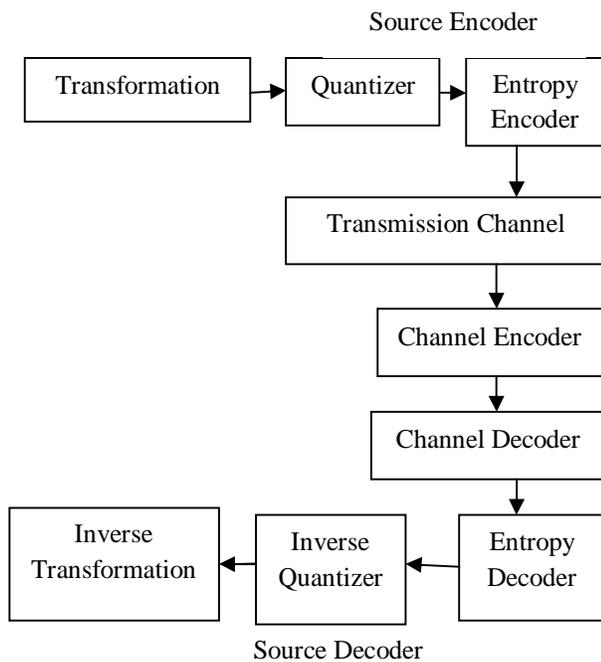
**Fig.2 Components of Typical Image/Video Transmission**
