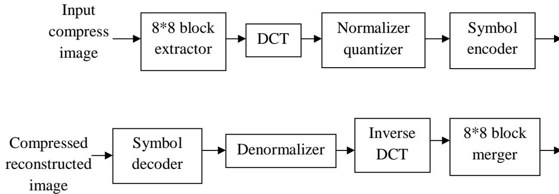
**Fig.3 image compression using DCT**
