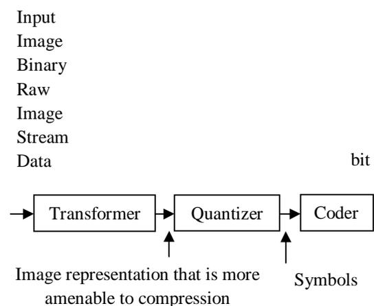
**Fig.1 Typical Image Compression System**
