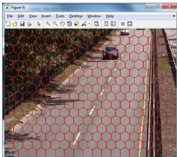
**Fig 5: Super pixel after thresholding**
