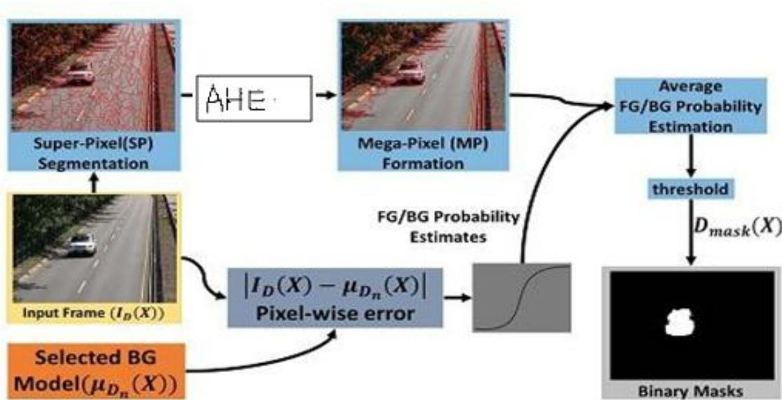
Fig 2: Binary Mask for Single Frame Using Adaptive Histogram Equalization
