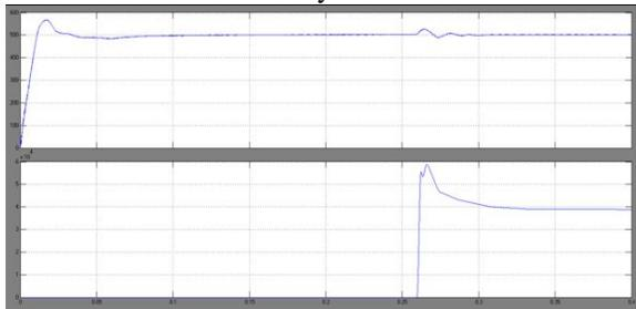
Fig.17. DC grid voltage and Real power delivered by SB
