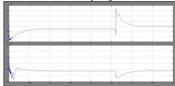
Fig.15. Real (top) and reactive (bottom) power delivered by inverter 1
