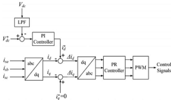
Fig.3.Configuration of the proposed controller for the ac/dc converter
