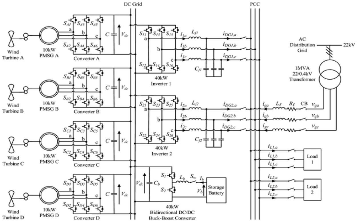
Fig.1. Overall configuration of the proposed dc grid based wind power generation system in a micro grid
