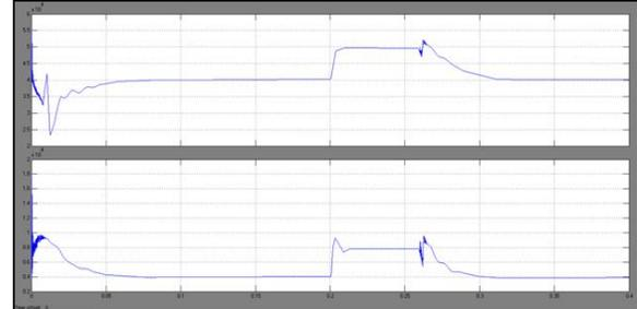
Fig.7. Real (top) and reactive (bottom) power delivered by the grid
