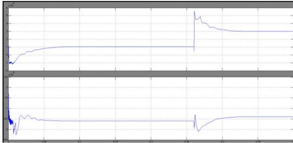
Fig.16. Real (top) and reactive (bottom) power delivered by inverter 2
