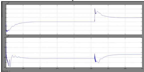
Fig.11. Real (top) and reactive (bottom) power delivered by inverter 2
