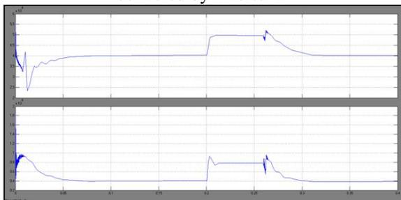
Fig.12. Real (top) and reactive (bottom) power delivered by the grid
