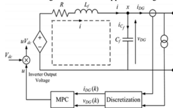
Fig.4. Single-phase representation of the three-phase dc/ac inverter
