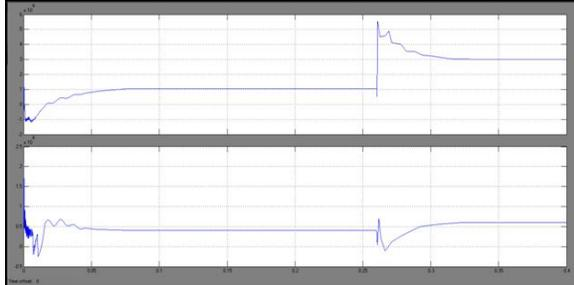
Fig.10. Real (top) and reactive (bottom) power delivered by inverter 1
