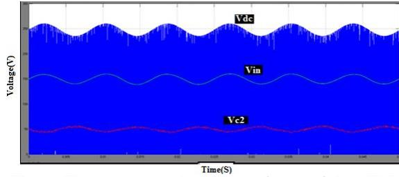
Fig. 8. The  $v_{DC}$ ,  $v_{IN}$  and  $v_{C2}$  waveforms of the qZSI with the conventional control,  $C_1=200\mu\text{F}$
