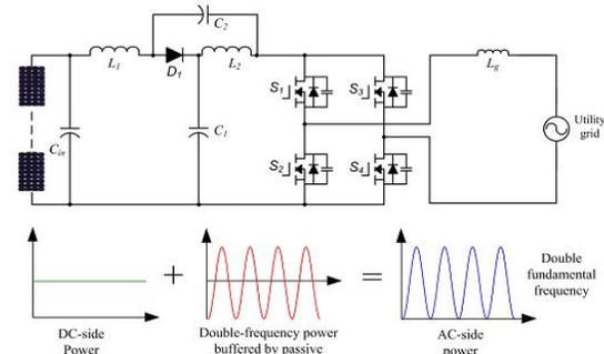
Fig. 1. Diagram of a single-phase qZSI based PV system.
