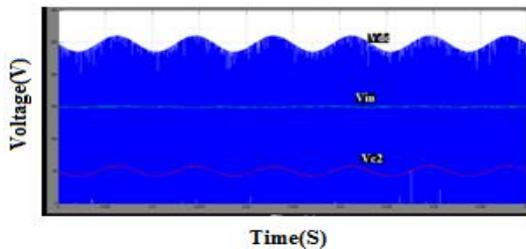
Fig. 9. The  $v_{DC}$ ,  $v_{IN}$  and  $v_{C2}$  waveforms of the qZSI with the proposed control,  $C_1=200\mu\text{F}$ .
