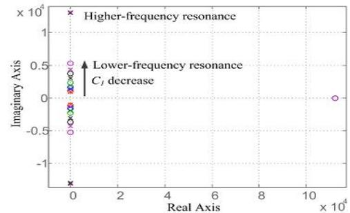
Fig. 4. Root loci of the system with C1 parameter sweeping.
