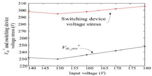
Fig. 5. V<sub>dc-ave</sub>\* and switching device voltage stress at different input voltages.
