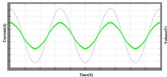
Fig. 10. The output current waveform of the qZSI with the proposed control,  $C_1=200\mu\text{F}$ .
