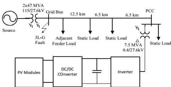
Fig. 1. One line diagram of the study system.
