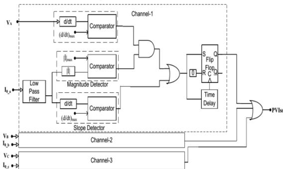
Fig. 3. Fault detection module
