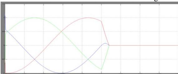
Fig. 6. (c) Inverter fault current with proposed fault controller
