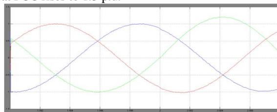
Fig. 7. (a) Inverter fault current at PCC during SLG fault at t = 2 second
