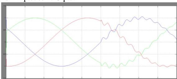
Fig. 6. (a) Inverter fault current at PCC during LLLG fault at t = 2 second
