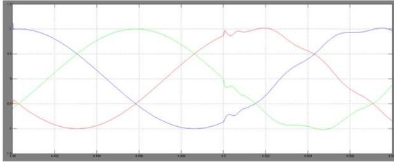
Fig. 6. (a) Inverter fault current at PCC during LLG fault at  $t = 4.5$  second
