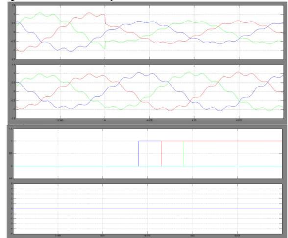
Fig. 11. Response of proposed controller for fast reclosure operation of relay.
