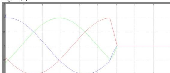
Fig. 7. (c) Inverter fault current with proposed fault controller
