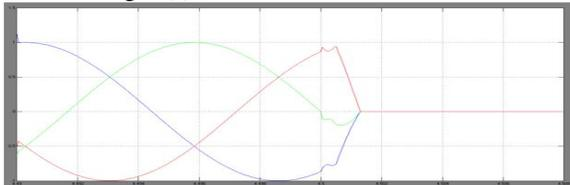
Fig. 8. (c) Inverter fault current with proposed fault controller
