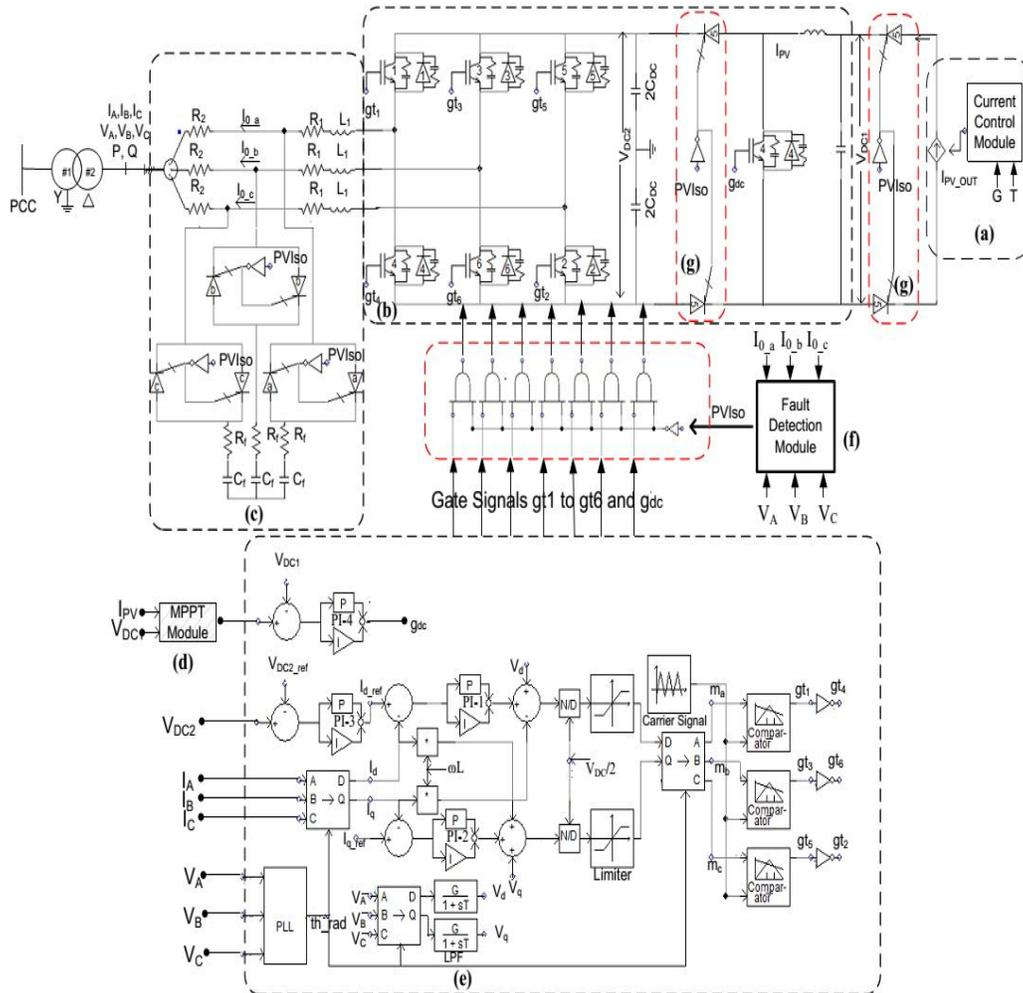
Fig. 2. Detailed PV system inverter and conventional controller with incorporated fault detection module.
