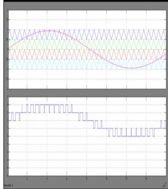
Fig. 2. Level-shifted multicarrier strategy for a five-level inverter. (a) Level shifted multicarrier modulation for a 5L FC-NNPC topology. (b) Desired output levels.
