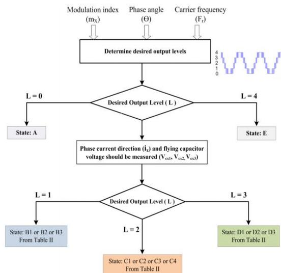
Fig.3. The procedure to control of flying capacitor voltages.
