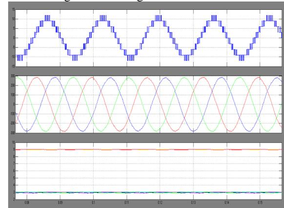
Fig. 9. Simulation waveforms in steady-state condition (a) inverter voltage, (b) output currents, and (c) voltages of flying capacitors ( $m=0.95$ ).
