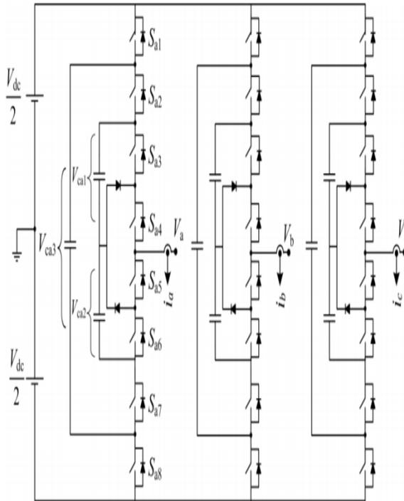
Fig. 1. A new five-level three-phase inverter.
