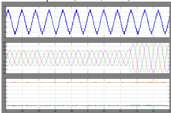
Fig. 12. Simulation waveforms in steady-state condition (capacitive load) (a) inverter voltage, (b) output currents, and (c) voltages of flying capacitors ( $m=0.9$ ,  $PF=-0.7$ ).
