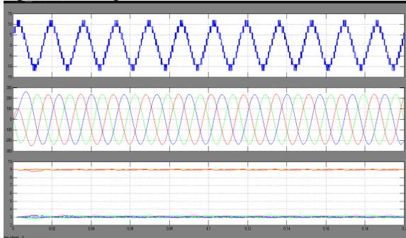
Fig. 10. Simulation waveforms in steady-state condition (a) inverter voltage, (b) output currents, and (c) voltages of flying capacitors ( $m=0.65$ ).
