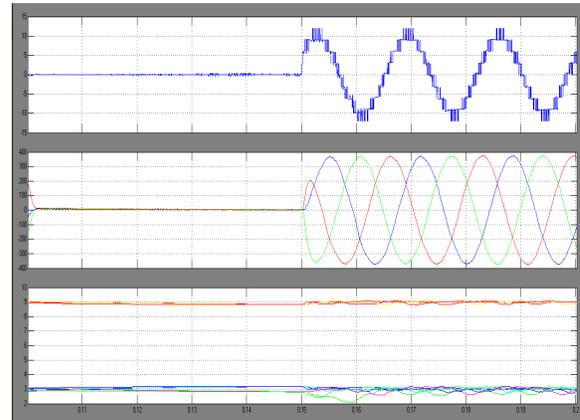
Fig. 13. Simulation waveforms in transient-state condition; load changes from half-load to full-load (a) inverter voltage, (b) output currents, and (c) voltages of flying capacitors ( $m=0.95$ ).
