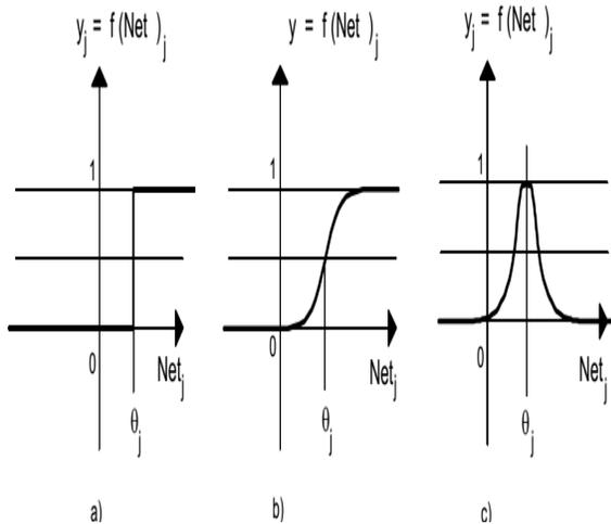
Fig. 6 Three different transfer functions: a threshold (a) a sigmoidal (b) a radial function (c) The parameter  $q_j$  in all three functions decides the  $Net_j$  value
