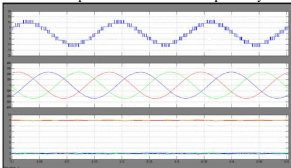
Fig. 11. Simulation waveforms in steady-state condition (inductive load) (a) inverter voltage, (b) output currents, and (c) voltages of flying capacitors ( $m=0.95$ ,  $PF=0.7$ ).
