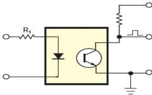
FIG: 3: Optocoupler structure
