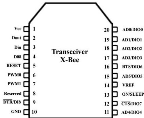
Fig .9: ZIGBEE pin diagram
