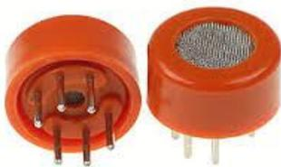
Fig.4: Alcohol sensor
