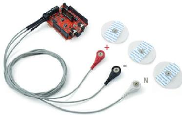
Fig .3: ECG Sensor
