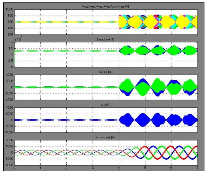
Fig 9. Simulation waveform when applying the conventional circulating current injection method with 6 r/min speed and step load torque from 10% to 36% of the rated torque
