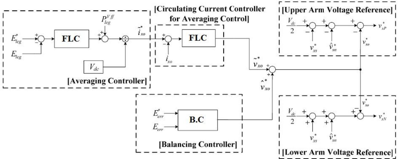
Fig.4. Proposed overall control scheme for variable-speed drives
