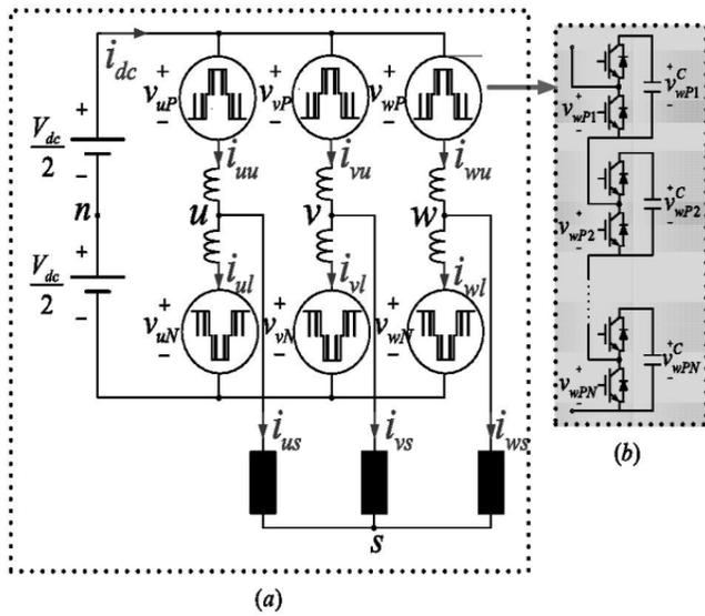
Fig.1. Circuit configuration of the MMC.
