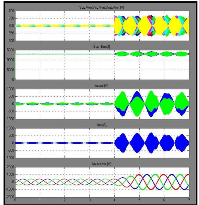
Fig. 8. Simulation waveform when applying the proposed leg offset voltage injection method with 6r/min speed and step load torque from 10% to 40% of the rated torque. (a) Sinusoidal waveform offset voltage injection (b) Square waveform offset voltage injection.
