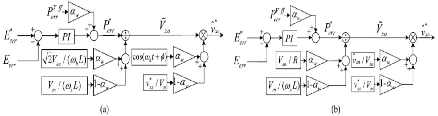
Fig.2. Proposed control scheme for variable-speed drives. (a) Sinusoidal wave voltage injection method. (b) Square wave voltage injection method.  $\alpha_w$  is weighting factor for switchover, which is described in Section III-C.
