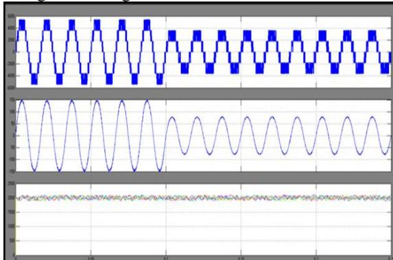
Fig. 5. Simulation results of NNPC inverter with SVM and the voltage balancing method for  $m_a = 0.8$  ( $t < 0.1$  s) and  $m_a = 0.5$  ( $t > 0.1$  s). (a) Line-line voltage. (b) Phase current. (c) Six FC voltages.
