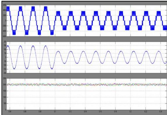
Fig. 4. Simulation results of NNPC inverter with SPWM and the voltage balancing method for  $m_a = 0.8$  ( $t < 0.1$  s) and  $m_a = 0.5$  ( $t > 0.1$  s). (a) Line-line voltage. (b) Phase current. (c) Six FC voltages
