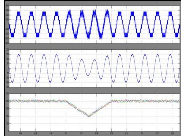
Fig. 6. Simulation results of NNPC inverter with and without the capacitor voltage-balancing control under SPWM scheme. (a) Line-line voltage. (b) Phase current. (c) Six FC voltages.
