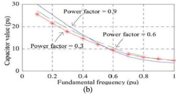
Fig. 9. FC value versus the inverter fundamental frequency with maximum peak-to-peak capacitor voltage ripple of 15%. (a) Fan/pump type of loads. (b) Constant torque type of loads.
