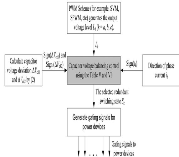
Fig. 3. Schematic diagram for integration of the proposed capacitor voltage-balancing method with PWM schemes.
