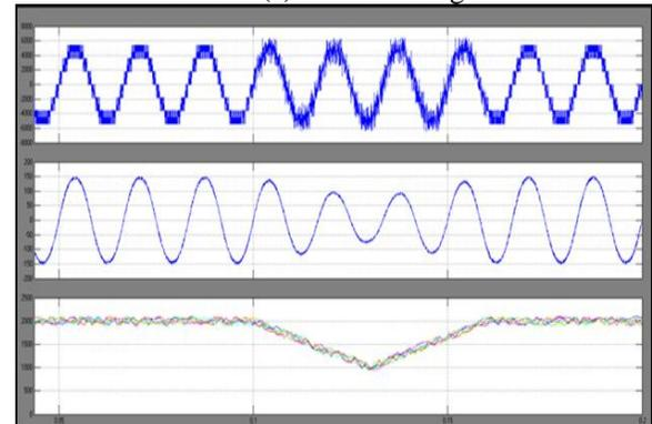
Fig. 7. Simulation results of NNPC inverter with and without the capacitor voltage-balancing control under SVM scheme. (a) Line-line voltage. (b) Phase current. (c) Six FC voltages.
