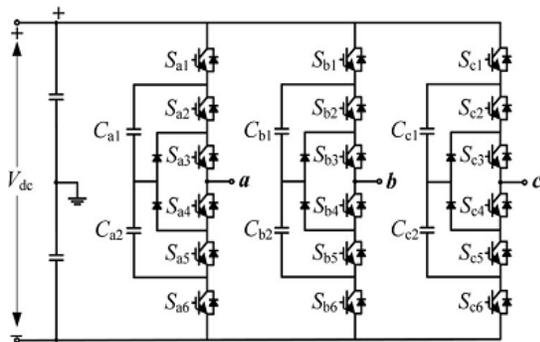
Fig. 1. Three phase nested neutral-point clamped (NNPC) inverter.
