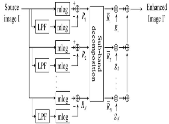
Figure 3: Block diagram of the conventional SD-MSR
