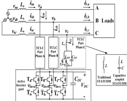
Fig. 1. Circuit configuration of the hybrid-STATCOM.
