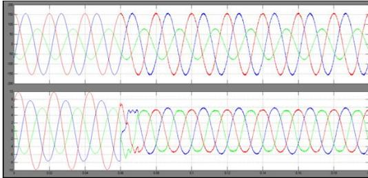
Fig10. Dynamic compensation waveforms of  $v_x$  and  $i_{sx}$  by applying hybrid-STATCOM under voltage fault condition.
