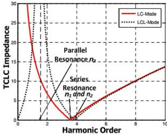
Fig4. TCLC impedance under different harmonic order.
