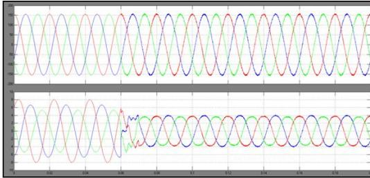
Fig9. Dynamic compensation waveforms of  $v_x$  and  $i_{sx}$  by applying hybrid-STATCOM under unbalanced loads.
