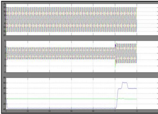
**Fig6.** Dynamic compensation waveforms of load voltage, source current, and load and source reactive powers by applying hybrid-STATCOM under different loadings cases.
