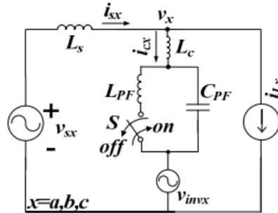
Fig3. Simplified single-phase equivalent circuit model of hybrid-STATCOM
