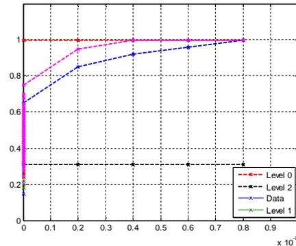
Figure .6. Illustration of the reduction ratio as a function of the channel gain being used to determine the allocating capacity for the NRT users
