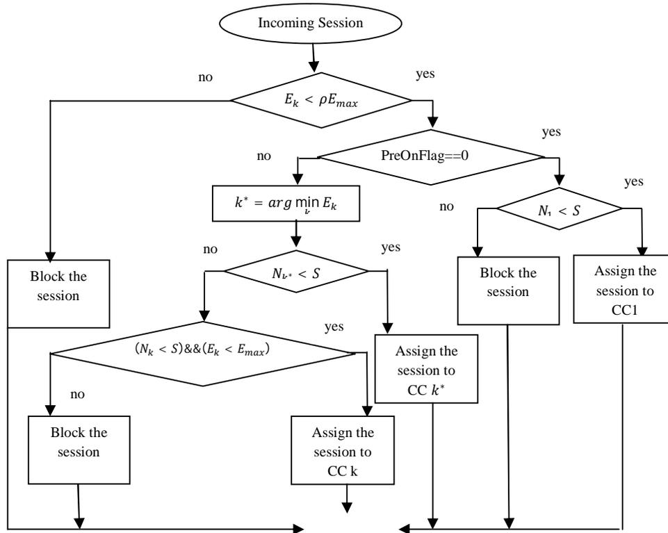
Figure 2: Flow chart of the admission control mechanism
