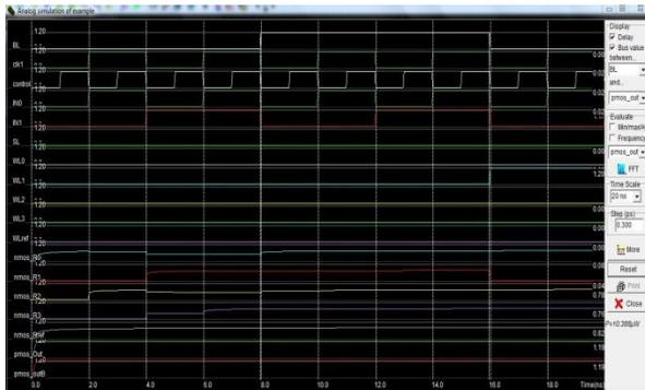
Fig 8. Voltage VS Time diagram for RRAM based two -input nvLUT.
