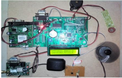
Fig.5.Main Circuit Board and CO Monitoring Equipment
