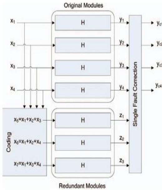
Fig. 1. ECC-based scheme for four filters and a Hamming code.
