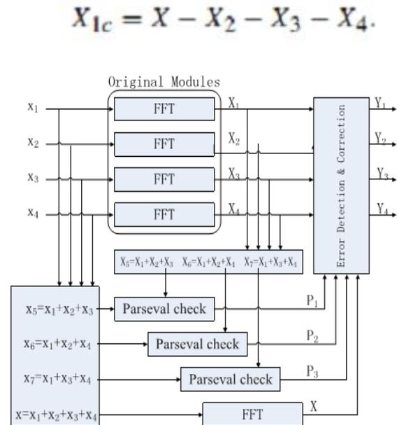
Fig. 3. Parity-SOS-ECC (second technique) fault-tolerant parallel FFTs.
