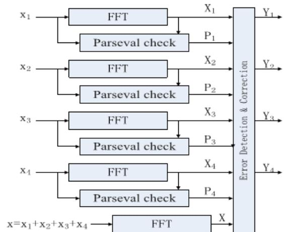
Fig. 2. Parity-SOS (first technique) fault-tolerant parallel FFTs.
