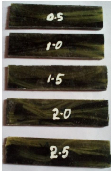
Fig 5 with addition of mild steel powder flexural specimens
