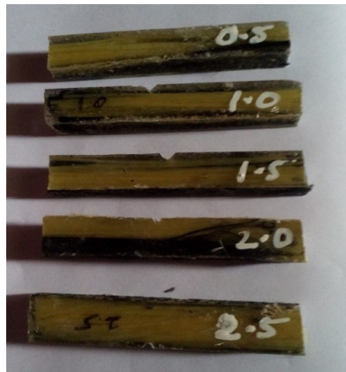
Fig 7without addition of mild steel powder impact specimen's
