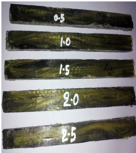
Fig 3 with addition of mild steel powder tensile specimens
