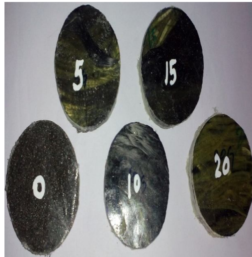
Fig 9 with addition of mild steel powder thermal conductivity specimen's
