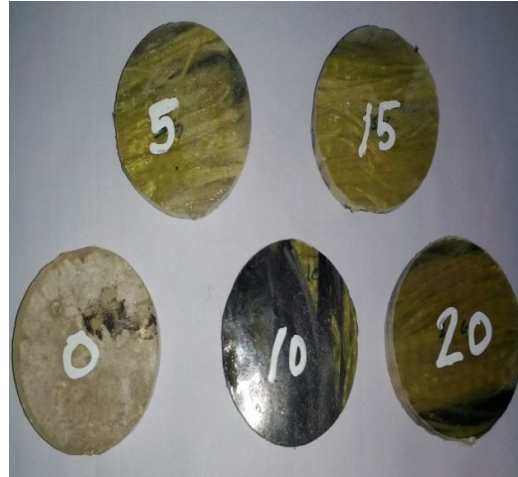
Fig 8 without addition of mild steel powder thermal conductivity specimen's
