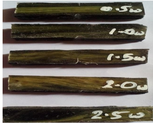
Fig 6with addition of mild steel powder impact specimen's
