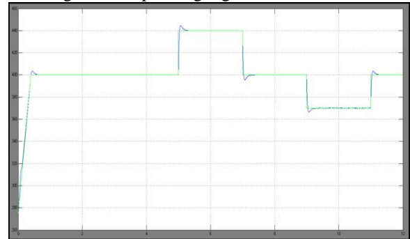
Fig.9. Simulation result for dc-link voltage v_C during step transient of its reference voltage with both step-up and step-down variations.
