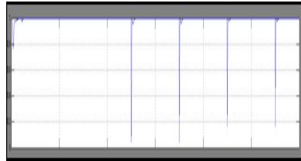
Fig. 14. Simulation result for function \mu used for commutation between the controllers P I and DSM – PI.
