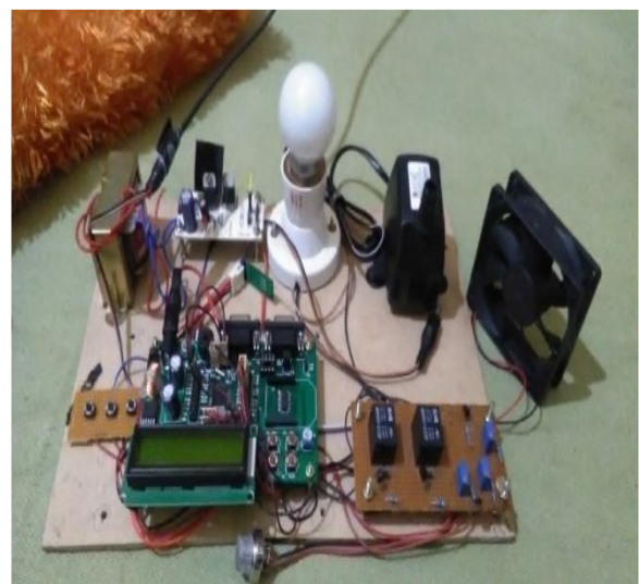
Figure 5: Hardware setup for receiver module
