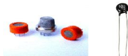
Fig 9: CO2 sensor, Temperature sensor
