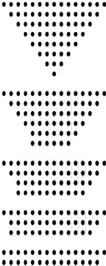
Fig.5: Example of Dadda reduction on 8x8 multiplier. Bits with lower weight are rightmost.
