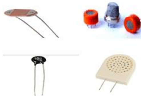
Fig 3: Sensors: a. LDR b. Gas c. Temp d. Humidity
